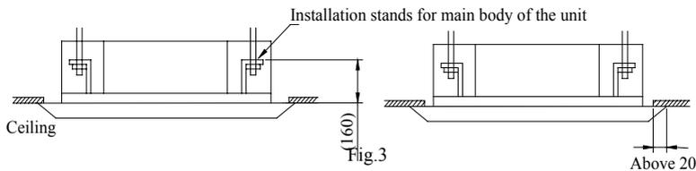
Notes: The dimension for the ceiling openings with \* marks can be as large as 910mm. But the overlapping sections of the ceiling and the decorated surface boards should be maintained at no less than 20mm.
